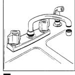
1 Turn on water supplies and check for leaks. With faucet off remove aerator. Turn on hot and cold to flush lines and faucet. Operate spray. Turn off faucet and replace aerator.
